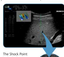
The Shock Point is the indication of shock and gate locations: useful to drive operator to select suitable measurement areas
