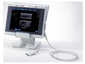
full touch screen technology, to onboard application libraries. Due to its flat front panel the MyLab<sup>TM</sup>One can be easily cleaned, allowing also the use of a dedicated cover for sterile environments.
