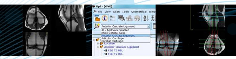
AgilExam automatically positions the slices both in terms of angulation and number according to the laterality and size of the anatomy under investigation.
