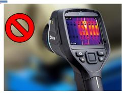
Infrared thermography: influenced by ambient factors (i.e. moisture, temperature)
