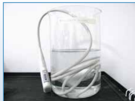
Figure 5 - Example of head and probe cable immersed in disinfectant
