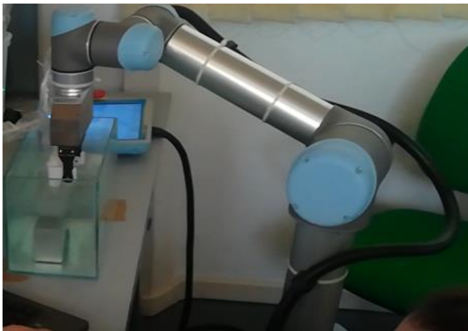
Fig. 7. UR5 with WSG performing an ECO pulse test.
