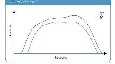
Figure 3 - Single Crystal (SC) provides up to 20-25% wider bandwidth and greater sensitivity compared to PZT. As a result, Doppler and tissue harmonic imaging per-
